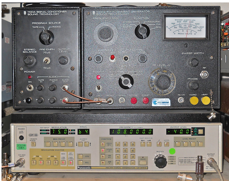
Figure 7. Panasonic VP-8191A generator fed by the Meguro MSG-211G-1; alternative setup with the ST1100A signal conditioner and the ST1000A FM alignment generator; both set for -40 dBm @ 108 MHz and 75 kHz deviation
