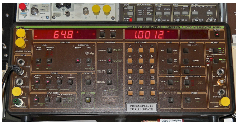
Figure 9. Amber 5500; THD measurement with bandwidth limiting of 400Hz and 30 kHz; output trimmer set for 500mV RMS at output; signal source set as per Fig. 7; input at Marantz 10B antenna terminal via a balancing transformer approximately -42 dBm
