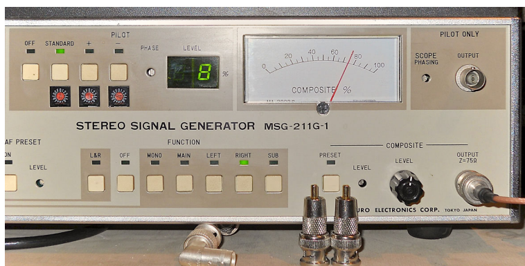
Figure 8. Meguro MSG-211G-1 as the main stereo encoder; Marantz 10B stereo measurement at 1 kHz with about 75% of the maximum allowable modulation, including 8% pilot tone
