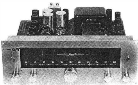
diodes, 7 indicator and voltage regulator neon tubes, and the cathode-ray tube for the scope. Circuitry and construction, in the Marantz tradition, are first-rate; high-grade parts are used; wiring layout is exemplary; workmanship is of the highest order. The tuning dial, measuring 10 $\frac{1}{8}$  inches across the 88-to-108-megacycle range, is unusually large and clear, and—with visible markings down to each 0.2 megacycle—permits accurate and precise tuning.
